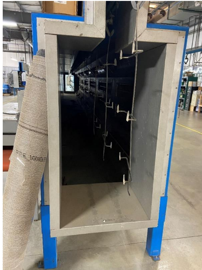
(Figure 1: The actual Infra-Red Oven I used to Re-heat these parts)
