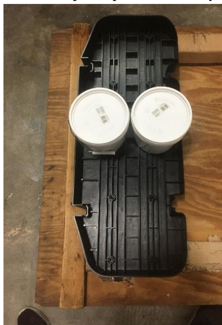
Figure 2 : Cooling Method with Weights to Prevent Warpage
