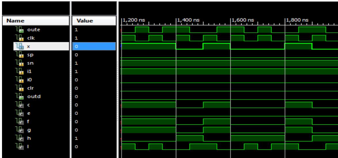
Fig.22. Simulation results of Manchester Encoding
