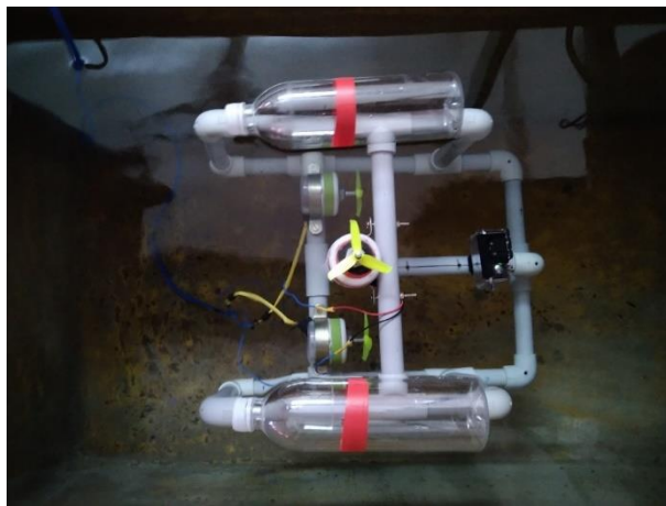
Figure 6. Experimental testing of the ROV (Surge)
