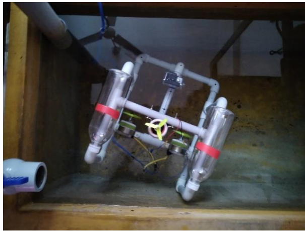
Figure 5. Experimental testing of the ROV (Sway)
