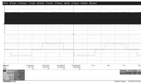
b. Waveform for the measurement Figure 4: Frequency dithering measurements
