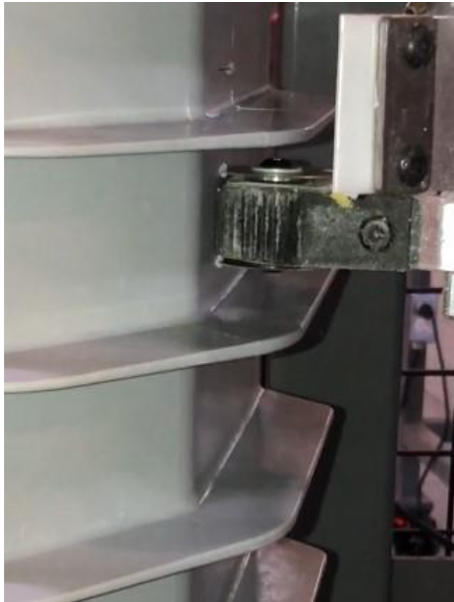
Figure 5: Final machined part with slots clean and free from flash and debris.
