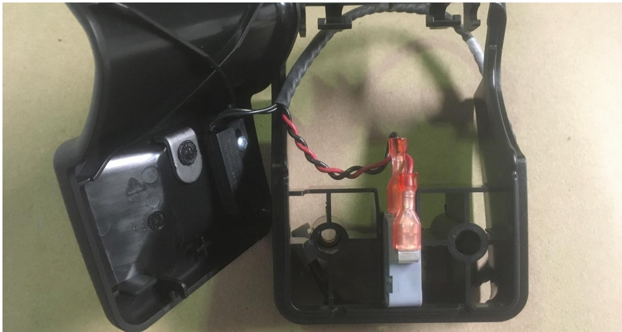
Figure 2: "Close-Up of Misaligned Wire-Harness Base"
