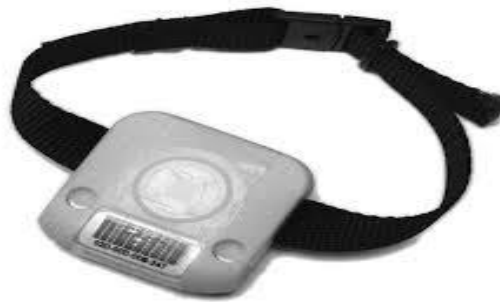
Fig.1. RTLS wristband with compact tag used in this study. It is both small and wireless, making it useful in this domain [7]
