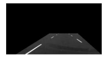
The low\_threshold, high\_theshold permit us to disconnect the nearby pixels that follow the most grounded angle. On the off chance that the slope is bigger than the upper edge then it is acknowledged as an edge pixel, on the off chance that it's underneath the low limit, at that point it is dismissed. On the off chance that the inclination is between the edges then it is acknowledged just if it's associated with a solid edge.
