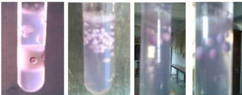
Figure 1 (a) Formation of halo in the precipitate; (b) growth conditions: Gel pH = 4.2, Conc. of upper reactant = 1M; (c) growth conditions: Gel pH = 4.2, Conc. of upper reactant = 0.75M; (d) growth conditions: Gel pH = 4.2, Conc. of upper reactant = 0.5M
