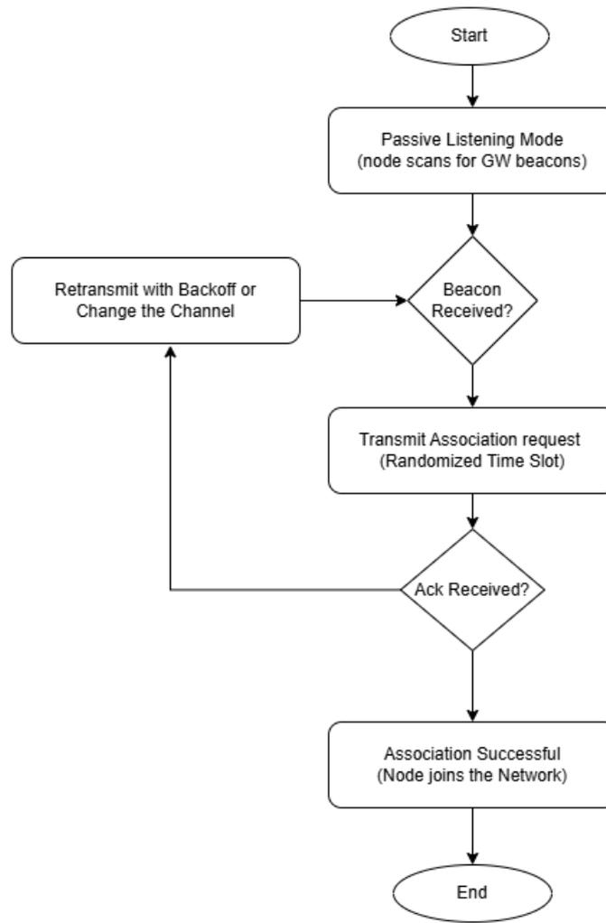
**Fig 1: Asynchronous Randomized Association Flowchart**
