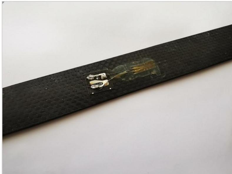
**Fig. 13** Tensile test specimen with strain gauge attachment
