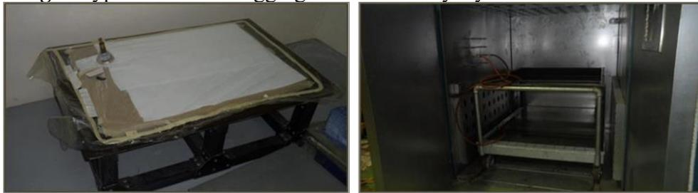
**Fig. 3** Vacuum Bagging Oven Cure (walk-in oven)
