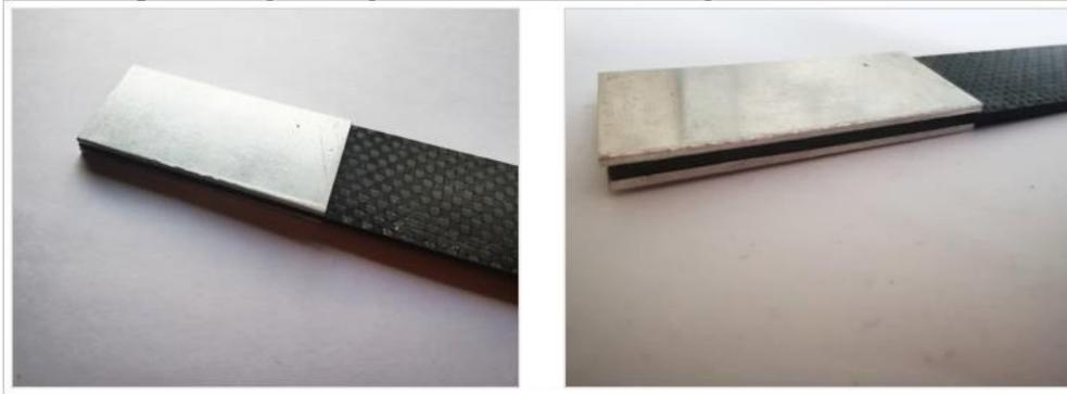
**Fig. 4** Aluminium end tab for carbon/epoxy composite tensile test specimen
