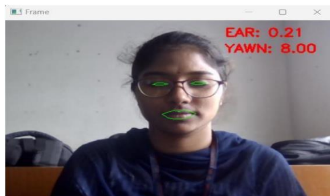
Fig 17 Output of Drowsiness Detection (closed eyes)
