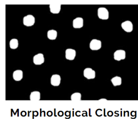
Figure 17: Applying morphological closing to the image
