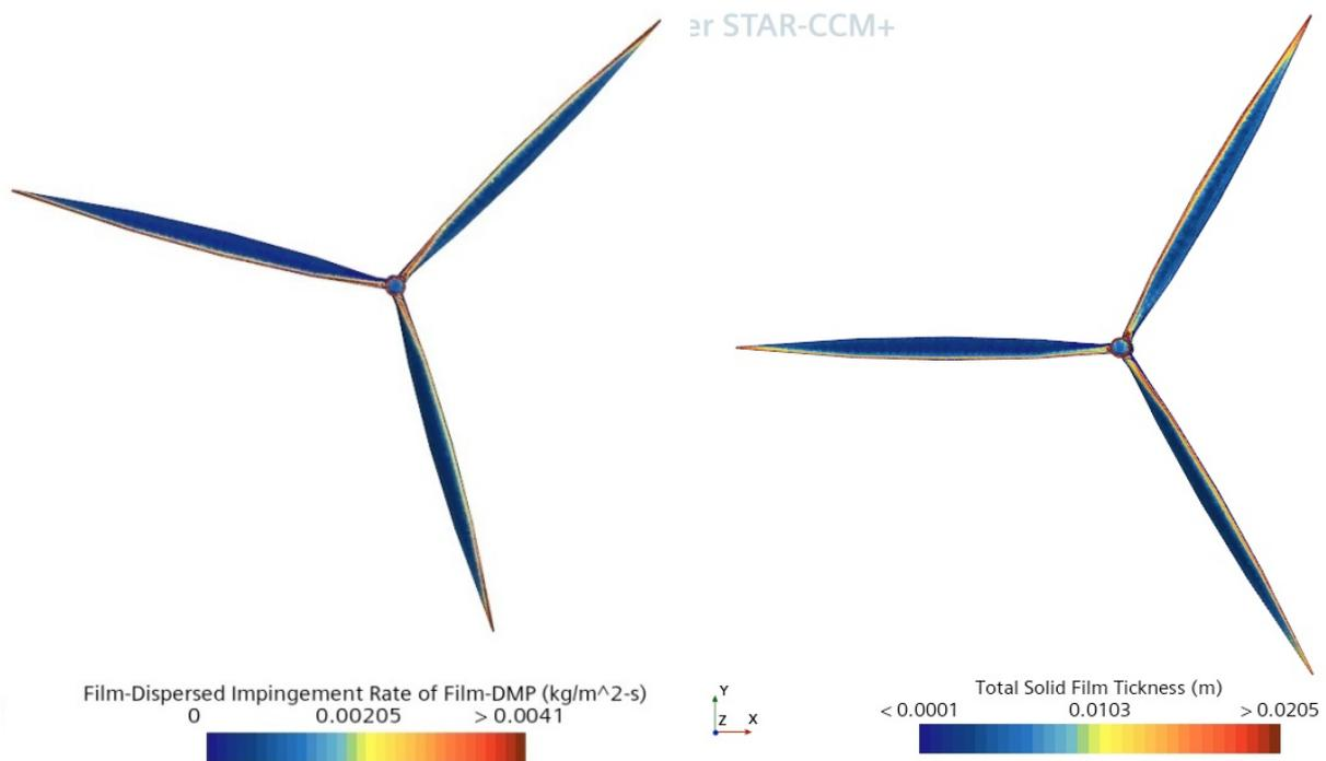
Figure 1: Results of modeling the icing process of wind turbine blades
