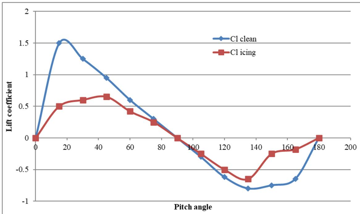
Figure 2: Blade lift coefficient with and without icing
